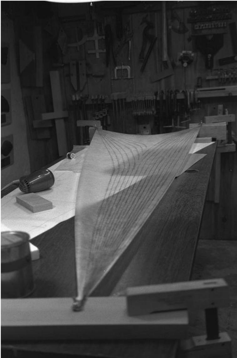
About three quarters of the threads, starting at the luff, are positioned at this point. Roughly half the threads terminate at the tack and the other half terminate at the clew. The threads from the head begin to arc towards their respective corners about two thirds the way down the sail. The threads are tacked down in these arcs 'freehand', by positioning the string with the Q Tip as it is glued. Use the previous thread as well as the position marks for a guide.
