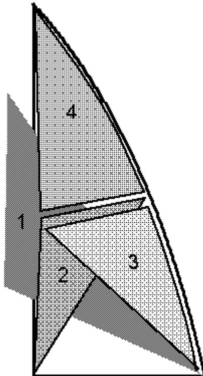
avoid snagging the filaments. The glue should be water thin. Glue only about five or six inches at a time to avoid sticking the threads down under tension. Make no attempt to keep the filaments straight. Just push them apart with your fingers so that they go this way and that, but in the general direction of the luff. Before the glue dries, you can further fan out the fibers. Try to avoid bunching them up with the brush.
