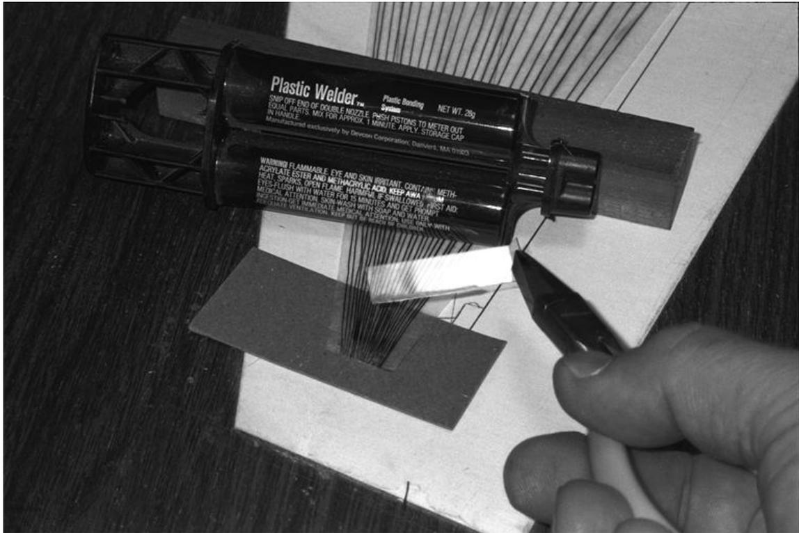
Now that all the threads are finally glued to the sail, the little tabs on the corners are cut off, leaving the sail at its final dimensions. At this point we need to evenly transfer the load on all the threads to the corner reinforcements. Here's how:
