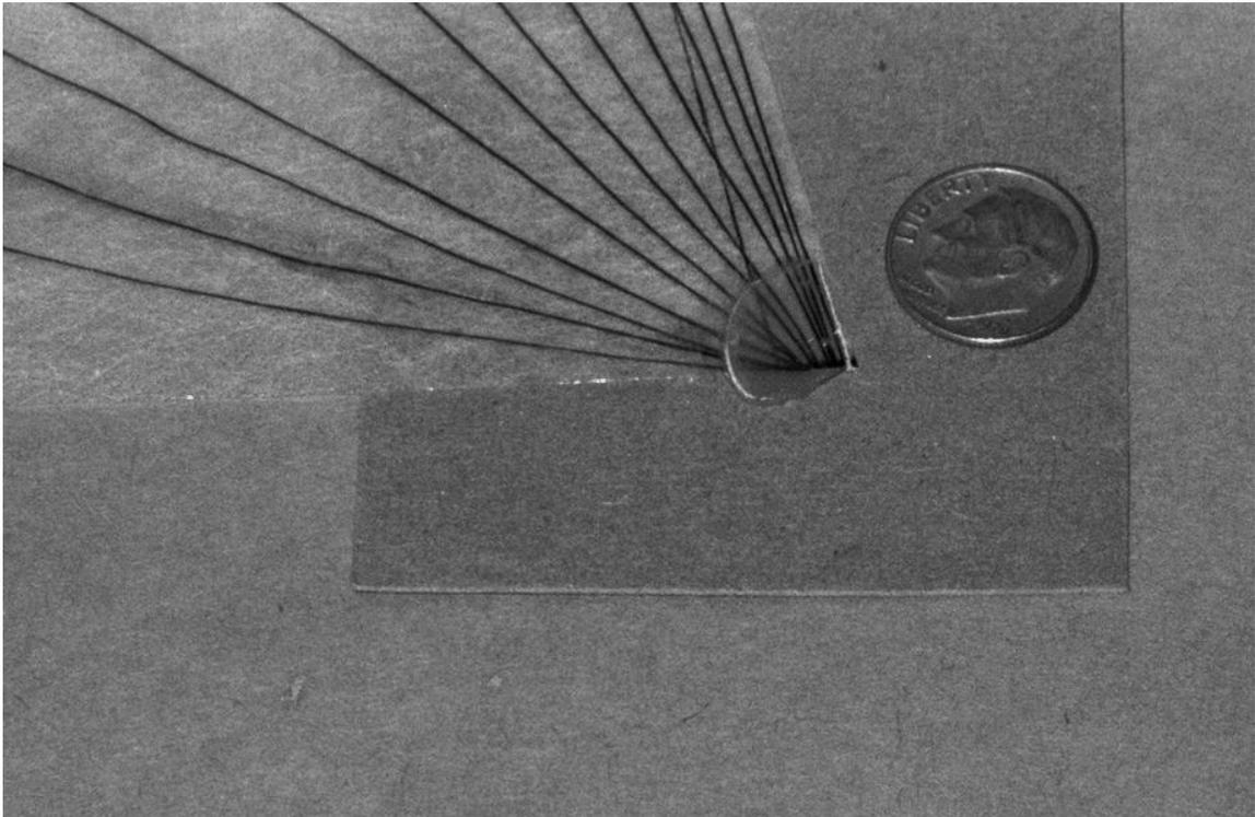
This photo shows the corner reinforcement at the tack of a jib. The tack of a main with a luff pocket would be made the same way. The sheet acetate reinforcement is attached in the same way as was done at the head. Although the small quarter circle of plastic has a radius of only about 3/8 inch, the result is amazingly strong. If done properly it's way in excess of working loads, as are the other corner attachments made this way.
