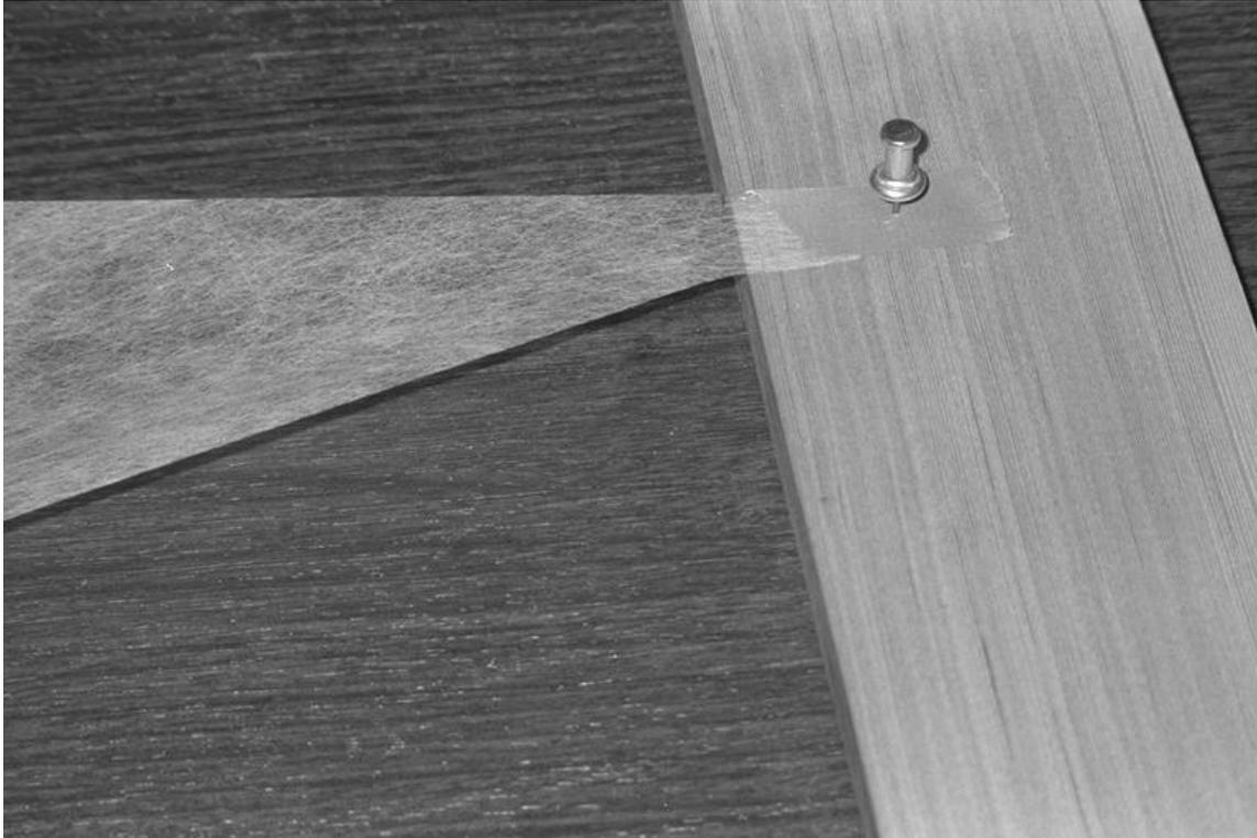
This photo shows in more detail how the head is temporarily pinned to the block (about 1 inch high) that supports it. Notice the small tab of fabric that projects beyond the final dimensions of the sail. A couple of pieces of masking tape stiffen the tab so that the push pin will not tear out.
