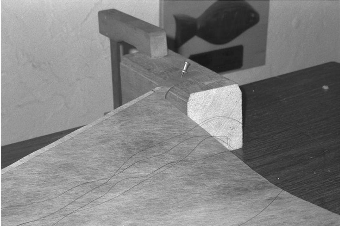
Photo 7 shows how the tack is supported, in this case for a jib. Note the luff pocket for the jibstay at the upper left. You can also see five strings draped along the sail, prior to their being glued in position. Support the clew in a similar manner.
