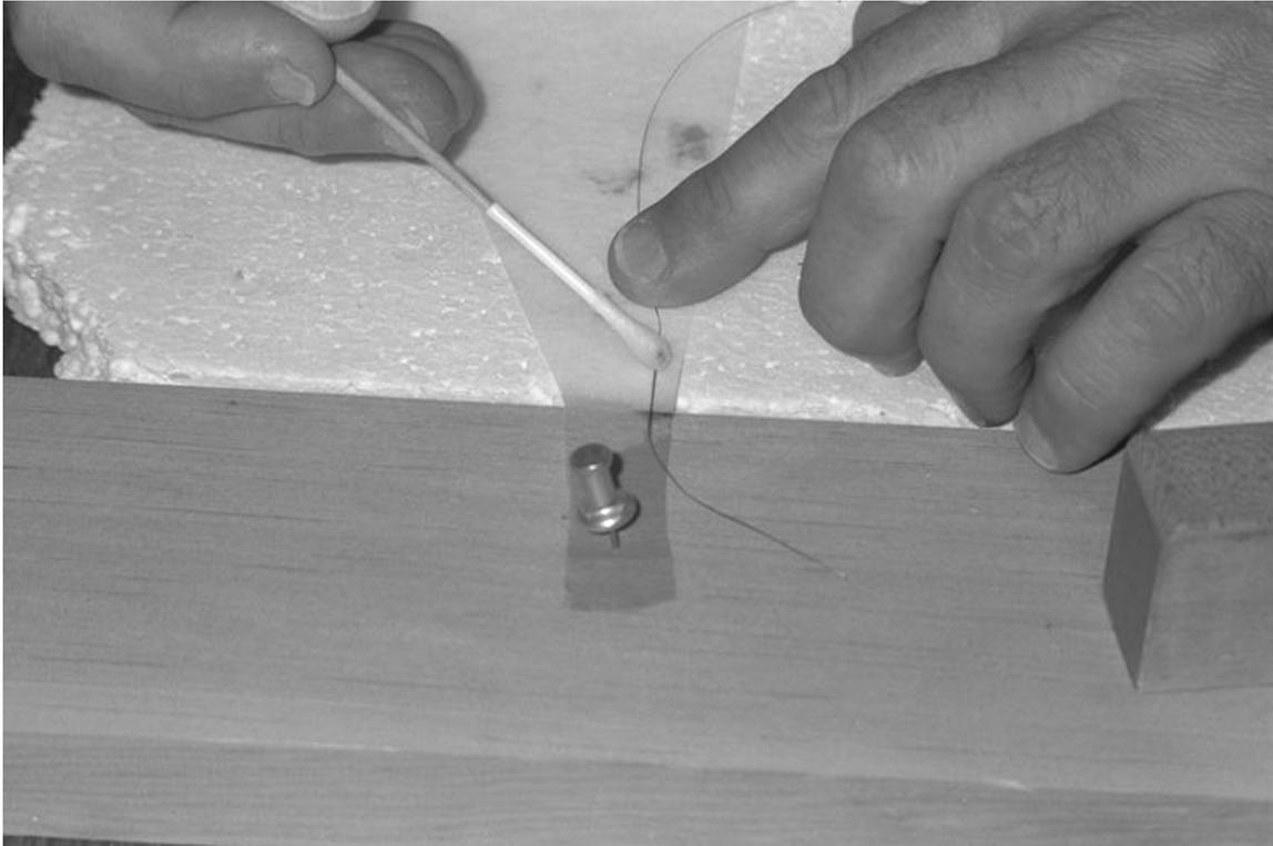
Here the first string is secured at the head, about 1/8 inch from the luff. The glue (described in the introduction) is applied with a Q-tip stuck on the end of a bamboo skewer. It gives better control than a brush. Only a half inch of string is stuck down at this point.
