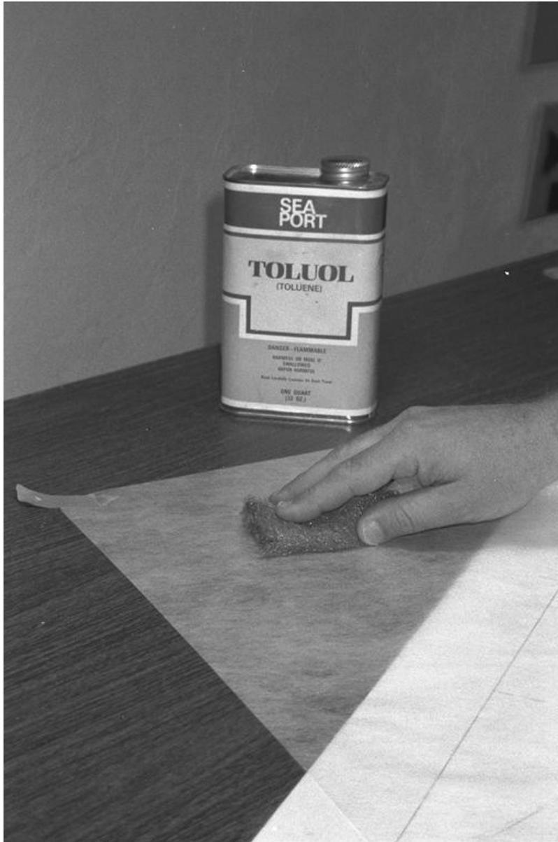
To help the threads bond to the shiny side of the clear Micafilm substrate, gently wipe the surface with steel wool and toluene. Don't scrub too hard or you will wrinkle the sail.
