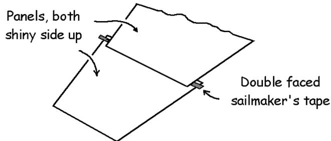
Therefore, the sail is made with the shiny surfaces of the panels facing all facing the same side of the sail. See **Figure 2**, compliments of Jeff Proulx.
