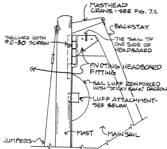
mast. Drill through the grommet and the hinge leaf while they are clamped together. Use a small drill bit (say 0.040 inches) to help keep the headboard in the proper place. (A large hole allows too much slop.)
