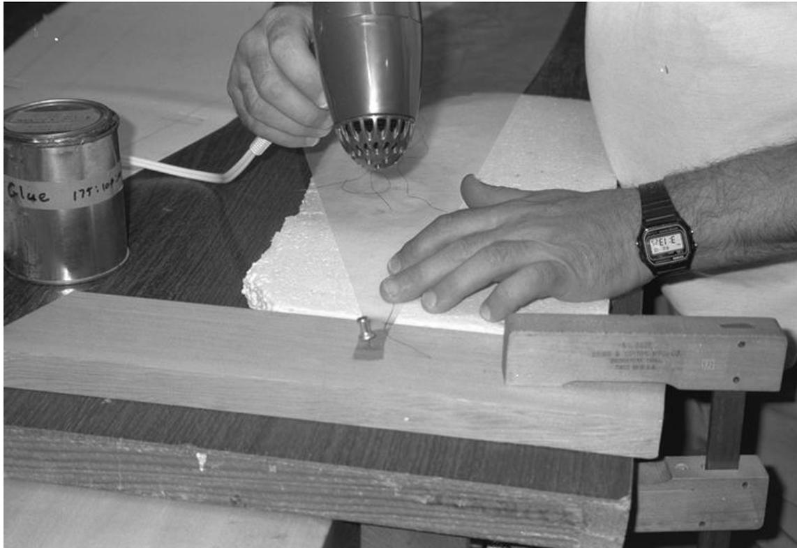
To save time, speed the drying of the glue with a hair dryer set on low. Be sure to test the dryer on a scrap of sail material first to make sure that it will not cause shrinkage. Here I am holding the thread down as the glue dries. Again, be aware of the potential danger from fire or explosion. Use adequate ventilation and assure yourself that the hair dryer is in good repair.
