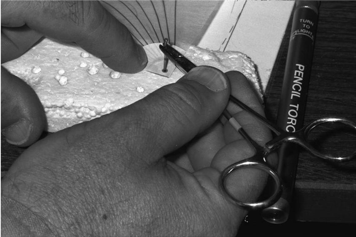
Photo 21 illustrates how to make the holes in the corner reinforcements. Metal islets are not necessary. Just heat an eighteen gauge brad with a torch and melt the holes as shown. I have never had one of these fail. If it were to happen I would regard it as a nice safety feature, in the same way as ‘D’ rings on full size jibs are sewn on in such a way that they may fail before the body of the sail fails.
