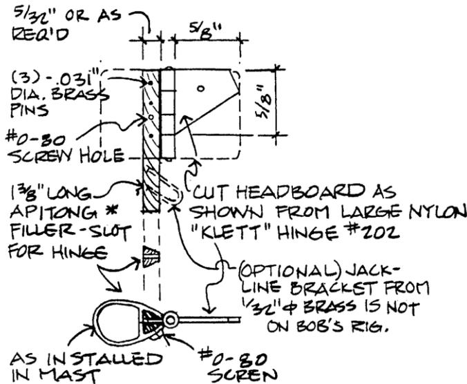
fitting shown in **Figures 1 and 2**. I suspect that there has not been a lot of interest in headboard attachment fittings to date because most EC-12 sails (as well sails made for other classes) are quite flat at the head. Hinging the headboard does not help a flat sail shape that much. However with the sails made using the ideas in these two sailmaking booklets (which suggest increasing the camber at the head) the sail will not set properly if this fitting is not used.
