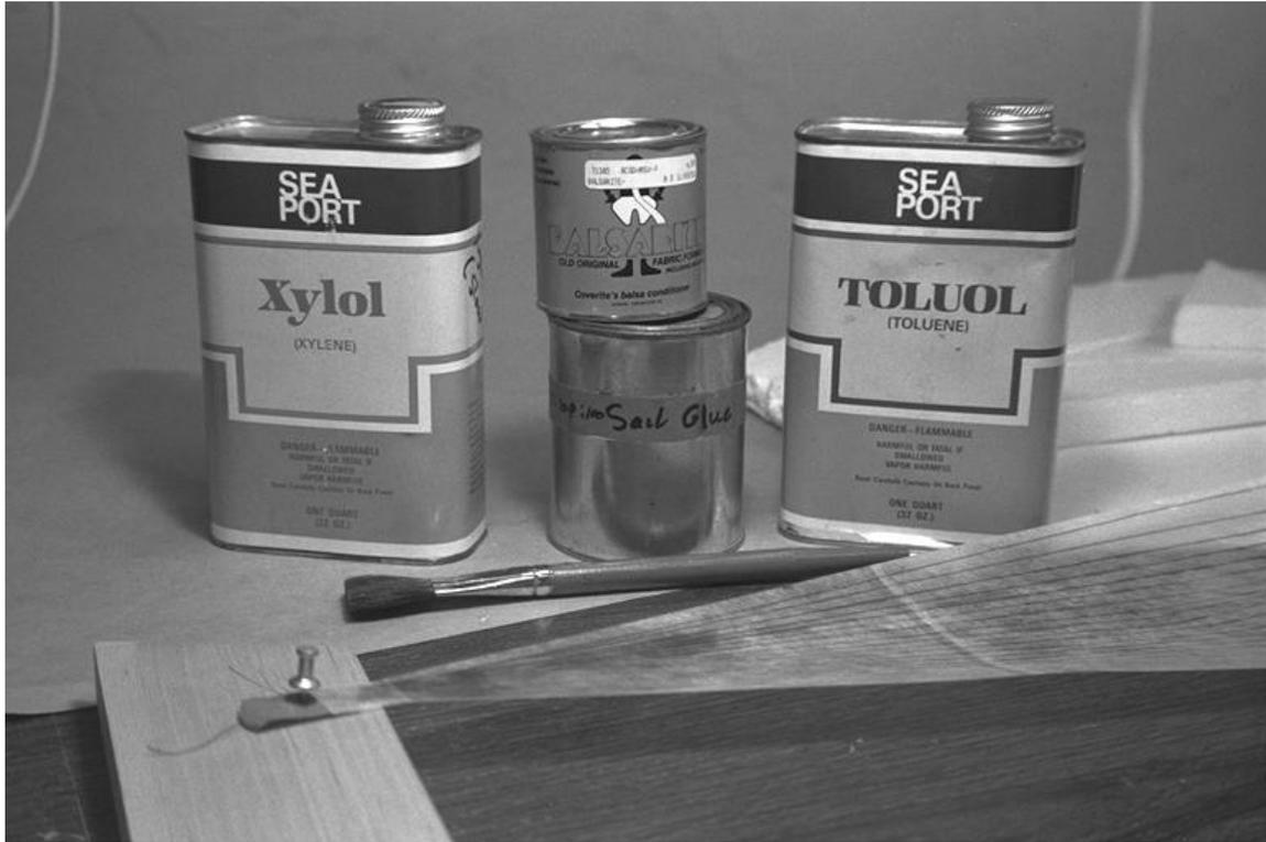
Some of the things that you will need are shown above. The most convenient work surface is your sail board. If you have not already made one, there is an article in the appendix on laying out the sail plan on the board. Here, a nearly finished sail is suspended above the board, pinned to blocks. There is more on this to follow. The strings are glued to the sail blank (shiny side to prevent curling) with thinned Balsarite. Use the original formula, No. 6000.
