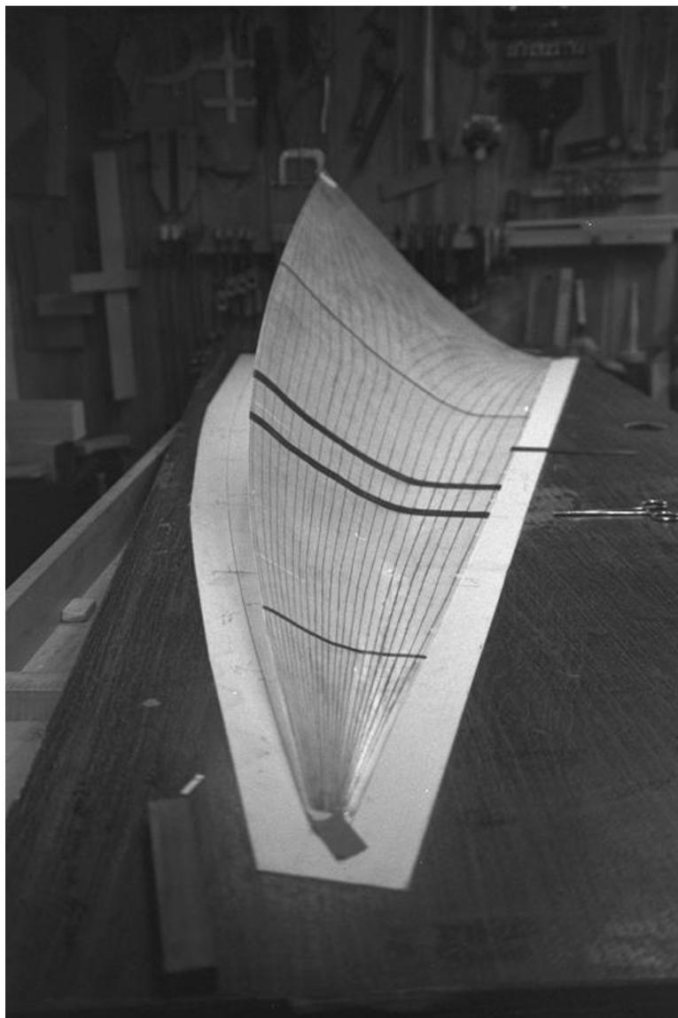
Here the mainsail has been finished. Draft stripes have been inked on with a permanent marker, and battens made of small strips of *MonoKote* have been applied. Because of the relatively small roach, EC-12 string sails do not benefit from typical stiff battens. Sails for classes that allow large roaches will require battens. I usually make them from sheet acetate and just stick them on with sailmaker's tape. (There is more on the subject in the Questions and Answers article in the appendix.)
