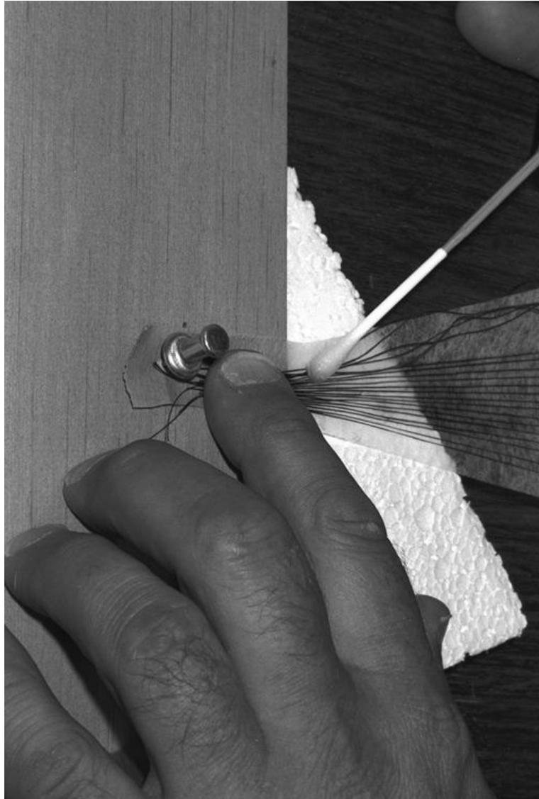
Here, three sets of five threads have already been applied from the head to the tack or clew of the sail. The last set of five is being stuck down at the head. (This sail will have 20 threads radiating from the head.) With practice, it's possible to glue two or three threads to the head at once, as shown here. The small foam block supports the sail as this is done.
